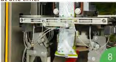
Special equipment forms a bag, doses a filling rate, compresses the contents and moves it further to be loaded on a pallet.
