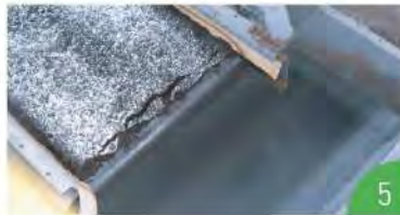
Screened peat and necessary additives are added according to the chosen formula and moved along the conveyor belt to the mixing line.
